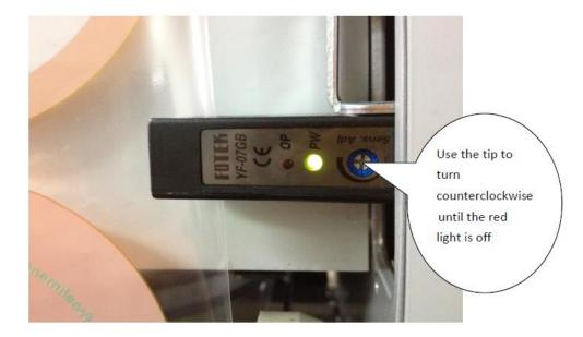
4) Only the green light should be on when the sensor is over the black eye-mark.
