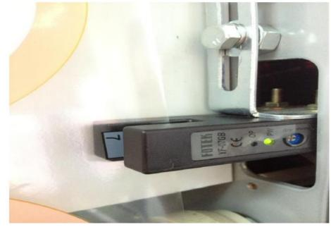
\*If the red light is on, this means the sensor is too strong. You can use the included tool below to adjust the sensor or a small Phillips head screwdriver.
