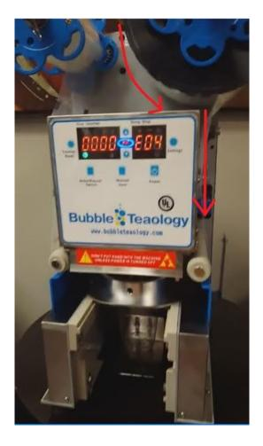
2) Please check the sensor and make sure the red light is off, this means it will detect the black "eye-mark".
