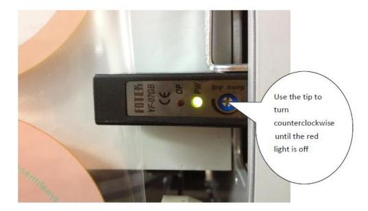
3) During normal use, only the red light changes. It will be off when it finds the black "eye-mark" and the red light will be on when no marks are present. This lets the machine know when to roll the film and when to stop it.
