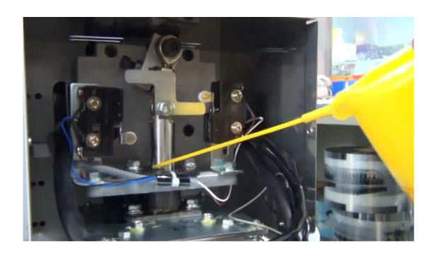
**Video - Lubricate Upper Mold Error E02**
