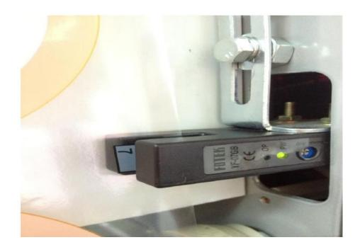
\*If the red light is on, that means the sensor is too strong. You can use the tool below to adjust the sensor.
