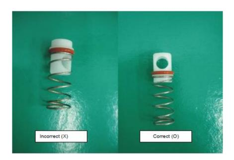
Sometimes if the plug head assembled incorrectly, the fructose will be blocked and cannot go out through the hole in the plug head.
